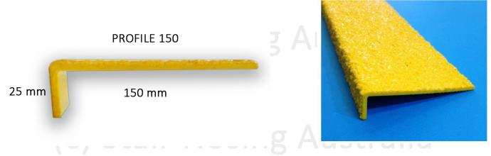
150 stair nosing has been slip resistance tested to AS 4586:2013 passing with the highest slip resistance rating of Class *P5* for Wet Pendulum Test and Class DI for Dry Floor Friction Test - LRV values on request
